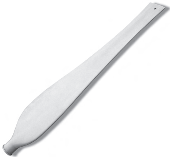
Figure 81 — Hollow-core fan blade.
